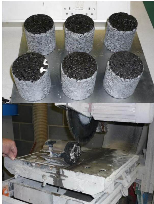
Picture 4-14 (a) Cylinders cored from specimen slab (b) slicing of cylinders
