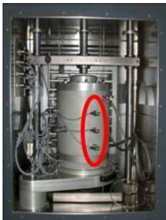
Picture 4-4 Position of the external LVDTs for the measurement of the radial or horizontal deformations (Grohs, 2005)
