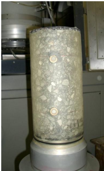
Picture 4-3 Position of the internal contact-less system for the measurement of the axial deformations (Grohs, 2005)
