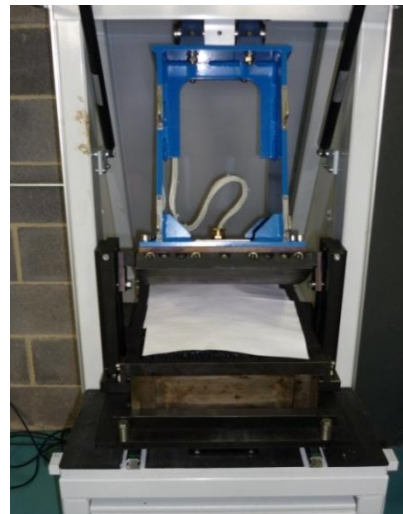
Picture 4-11 Samples placed in roller compactor (sheets of paper used to prevent material sticking to roller)
