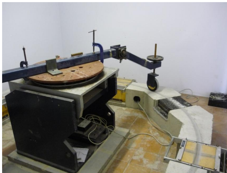
Picture 8-1 UCD circular wheel tracker - redesigned track
