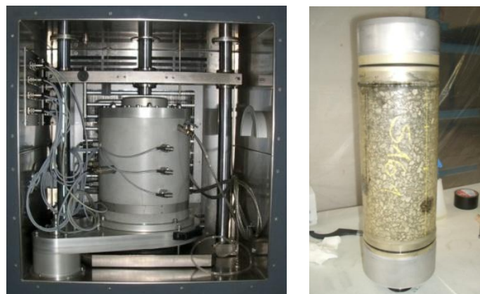
Picture 4-2 Triaxial pressure cell and specimens covered by a rubber membrane
