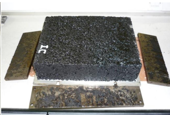
Picture 4-12 (a) Compacted specimen slab (b) Compacted specimen slab with steel mould removed
