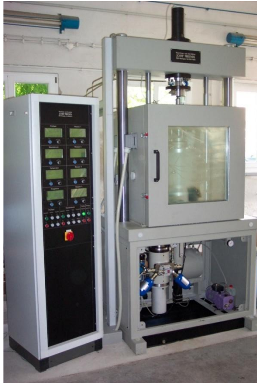
Picture 4-1 Repeated load triaxial test machine with a triaxial pressure cell at TU Dresden
