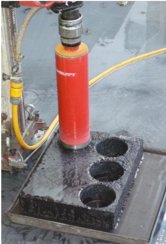
Picture 4-13 Coring of cylinders from specimen slab
