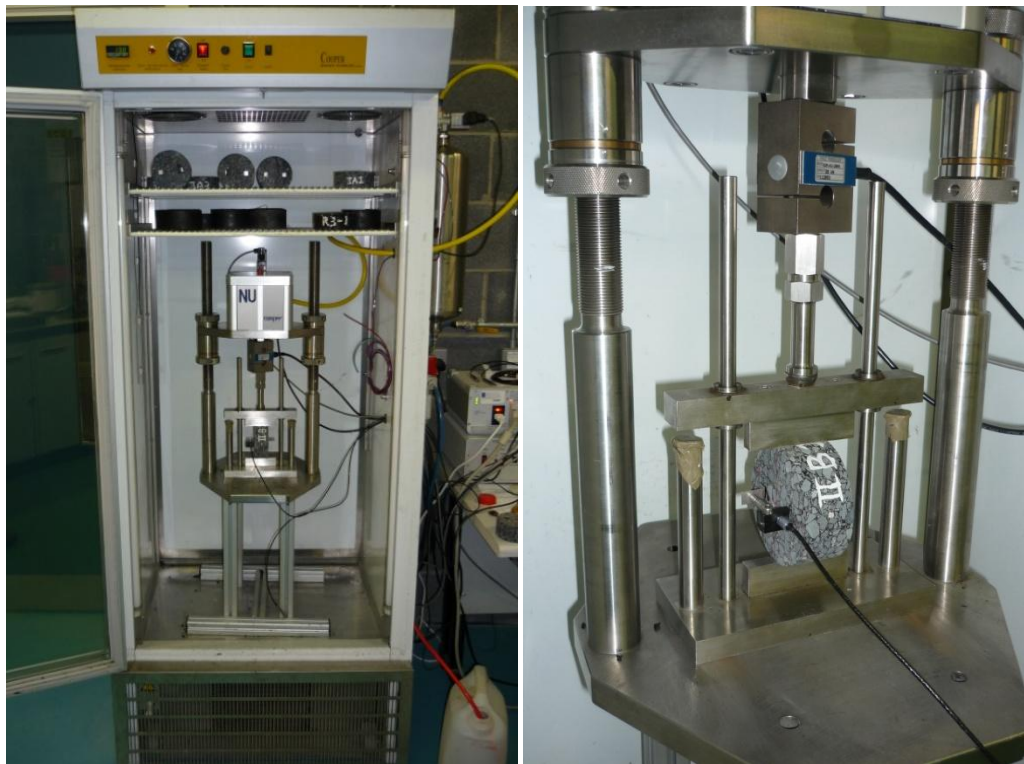
Picture 4-16 Cooper Technology Servo-Pneumatic Universal Testing Machine NU-10 testing apparatus in temperature controlled cabinet
